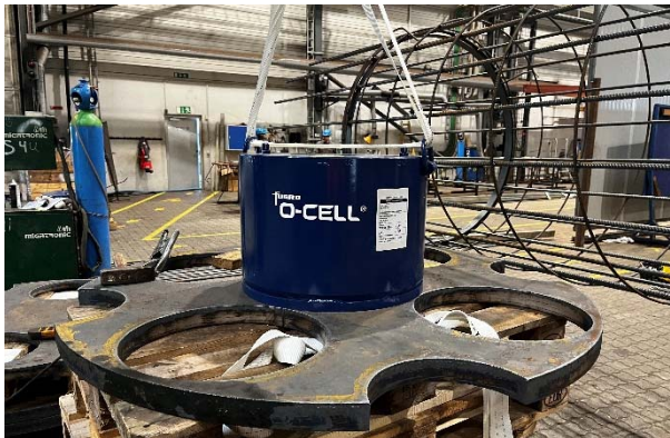
O-Cell assembly preparation and installation
